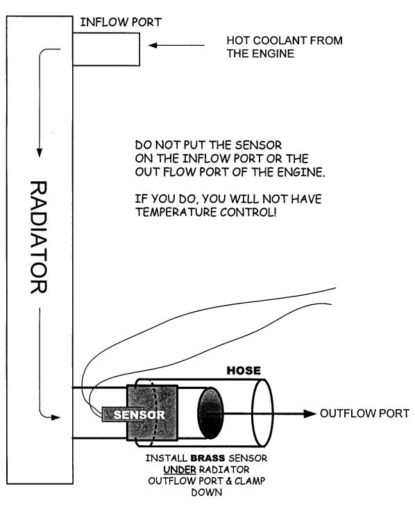
SENSOR RESISTANCE CHECK; 40,000 - 60,000 OHMS COLD OPEN FROM LEADS TO BRASS
